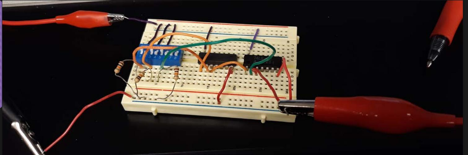
Step 3: Create the simulation in the lab to compare the results. The data sheets were used as references to wire the AND/OR gates. We used the same set up for each type of circuit then just switched the gates for the same wiring.
